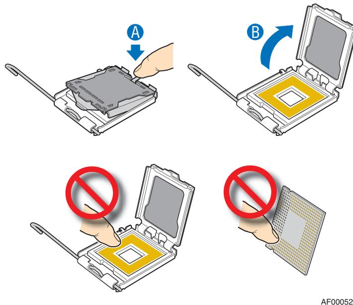
**Figure 23. Opening the Load Plate**
