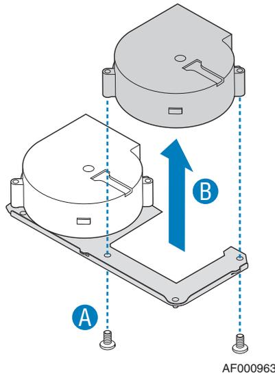
**Figure 74. Removing Fan from Fan Bracket (SR1530SH)**
